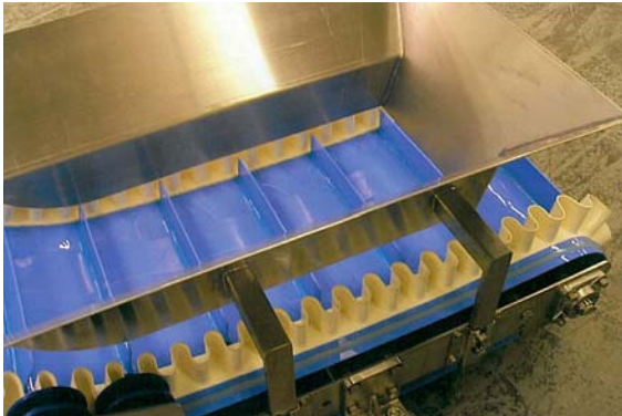
Hopper- Cleated Belts w/ Accodian Side Walls
