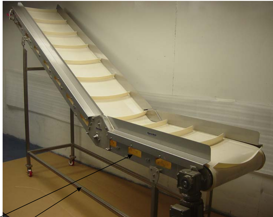
Hoppers, top covers, drip pans and multiple belt options including perforated belts. Cleats and Accordion Side Aprons to 4.5" Tall
