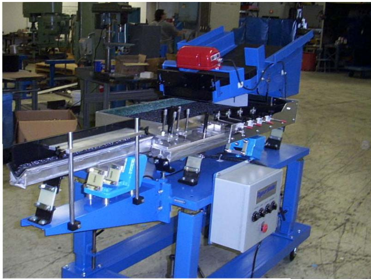
Live Pan w/ active pan for unloading customer's front dump container. Container has end gate which controls part escape.
