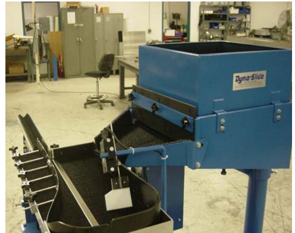
Live Pedestal Hopper w/ Brushed Pan Buffer Supply to 929 Part Feeder
